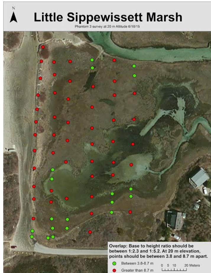
Figure 3. Map showing unsuccessful survey of Little Sippewissett Marsh. Not enough overlap was captured at a 20 m elevation resulting in poor image alignment in PhotoScan.
