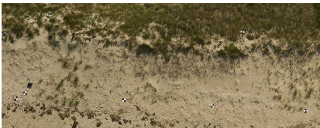
Figure 4. Image showing well-distributed GCPs (black and white targets) placed throughout the survey area.
